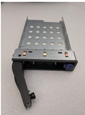
Figure 2.7: Assembled DiskTray
